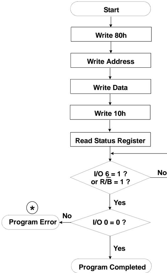
**\*** : If program operation results in an error, map out the block including the page in error and copy the target data to another block.
