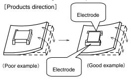
The electorode part of the products should be located like the picture to the mechanical stress.
