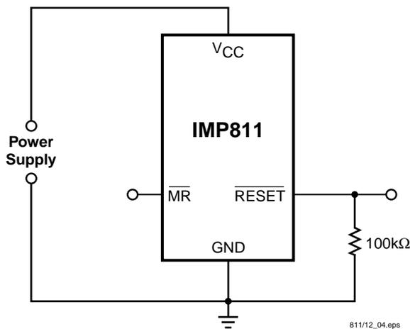
Figure 2. RESET Valid with  $V_{CC}$  Under 1.1V
