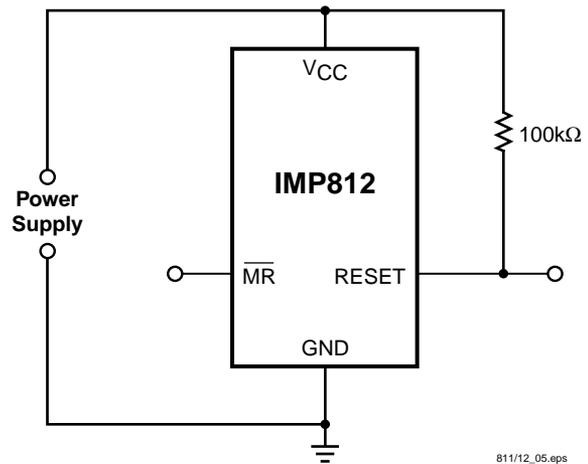
Figure 3. RESET Valid with  $V_{CC}$  Under 1.1V
