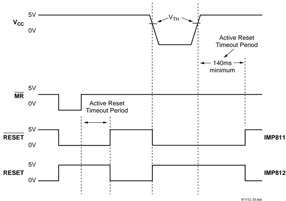
Figure 1. Reset Timing and Manual Reset (MR)
