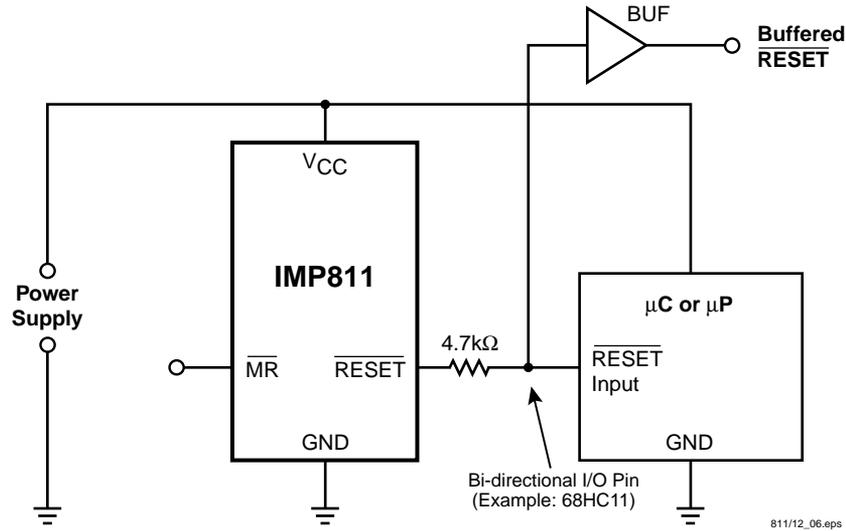
Figure 4. Bi-directional Reset Pin Interface
